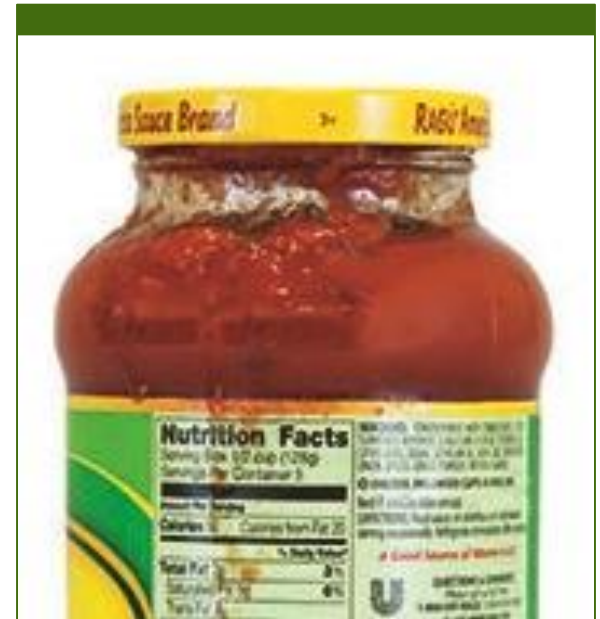
Signs of leakage
